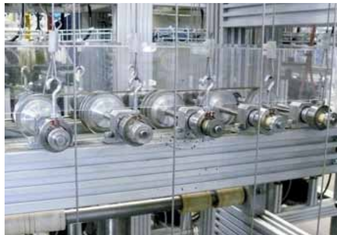
Test bench for xiros® polymer ball bearings at igus® laboratory
