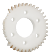
POM 621,000 cycles Failed
